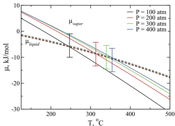
FIG. 8. Projections of the  $\mu(P, T)$  surfaces onto the  $\mu - T$  plane for various pressures showing the intersections which determine the coexistence line. The error bars indicate approximate numerical uncertainties, which arise mainly from the simulations of the chemical potential of the vapor phase.
