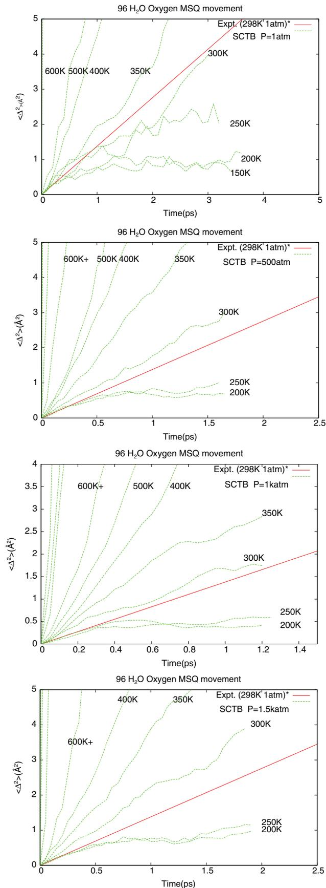
FIG. 10. Mean square displacement of water molecules in as calculated at various temperatures and pressures in the SCTB model with 96 water molecules. The red lines are obtained from the experimental value of the diffusion constant at 1 atm and 298 K.
