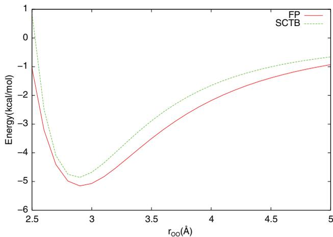
FIG. 2. Energy of the water dimer as a function of the oxygen-oxygen distance after the fit.
