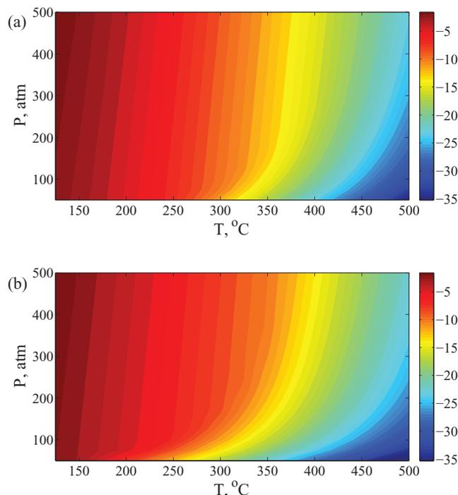
FIG. 7. Experimental values (a) and calculated values for the SCTB water model (b) of the chemical potential as a function of temperature and pressure. For the SCTB model, only the chemical potential for the phase with the lowest value of the chemical potential at a particular temperature and pressure is shown. The color intensity scale is in units of kJ/mol in both figures.
