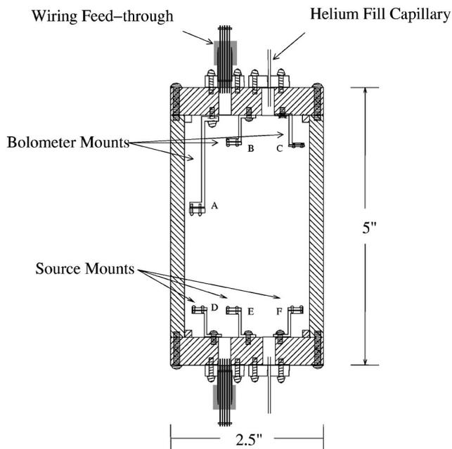
FIG. 1. Experimental cell used in the dilution refrigerator for vapor propagation experiments in the absence of a suspended film. The data reported in this paper were obtained with source *E* and bolometer *B*.
