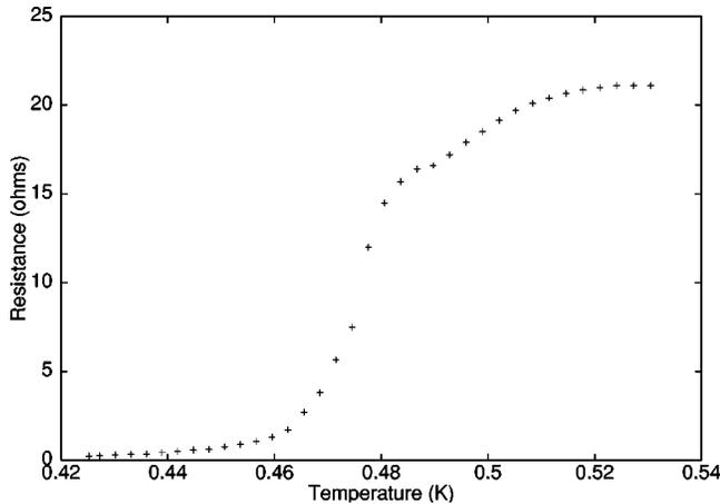
FIG. 2.  $R$  versus  $T$  for a titanium bolometer.
