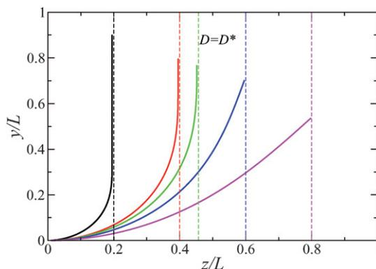
**Fig. 1** The equilibrium shape of a rod of length,  $L$ , for various wall separations,  $D$ , as determined by minimization of the bending energy, eqn (9), under the constraint of eqn (10) and the condition that the chain emerges perpendicularly from the wall, located at  $z = 0$ , on which it is grafted. Note the change in the conformation when the threshold value  $D = D^*$  is crossed.
